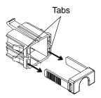
(2) With the main unit display part positioned so that it is facing down, attach the USB holder to the USB host interface. Do this by inserting the picks on the USB holder itself into the attachment holes on the main unit. Insert the upper hook first.
