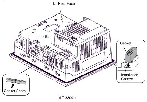
(4) Check that the gasket is attached correctly to the LT.
