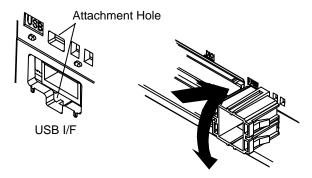
(3) Insert the USB cable into the USB Host Interface.
