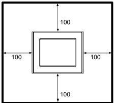
Be sure that the surrounding air temperature and the ambient humidity are within their designated ranges. (Surrounding air temperature: 0 to 50°C, Ambient humidity: 10 to 90%RH, Wet bulb temperature: 39°C max.) When installing the LT on the panel of a cabinet or enclosure, "Surrounding air temperature" indicates both the panel face and cabinet or enclosure's internal temperature.
