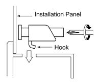
(3) Insert each of the fasteners shown below. Be sure to pull the fastener back until it is flush with the rear of the attachment hole.
