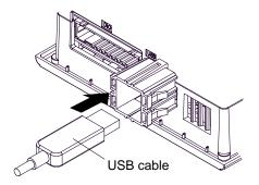
(4) Attach the USB cover to the USB host interface. Insert the USB cover into the tab of the USB holder.
