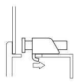
(4) Use a Phillips screwdriver to tighten each fastener screw and secure the LT in place.
