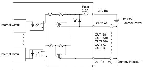
\*1 (Example) The output delay time (ON to OFF) is 1.5μs where the output current is DC 24V, 50mA. Install an external dummy resistor to increase the amount of current when more responsiveness is required and the load is light.
