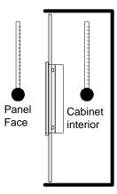
Be sure that heat from surrounding equipment does not cause the LT to exceed its standard operating temperature.
