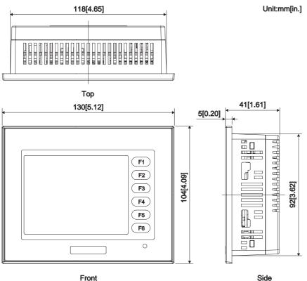
The following drawing shows the ST unit with installation fasteners.
