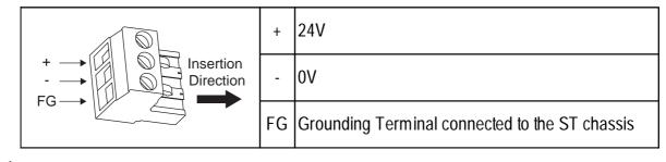
Note: The power cord should be equivalent to the specification shown above. Be sure to twist the power cords together, up to the power plug. (See illustration on next page)
