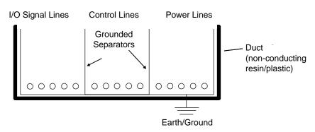
**NOTE** • If the lines cannot be separated, use shielded lines and create a ground from the shield line.
