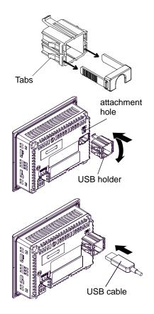
(4) Attach the USB cover to fix the USB cable. Insert the USB cover into the tab of the USB Holder.
