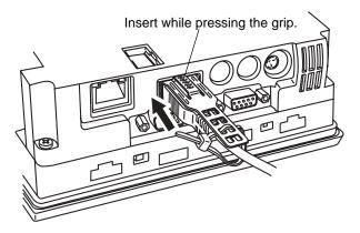
(5) As shown, completely tighten the tie and thoroughly attach the clip on the connector shell.
