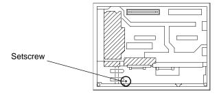
(5) Open the circuit board chassis, lifting from left to right.
