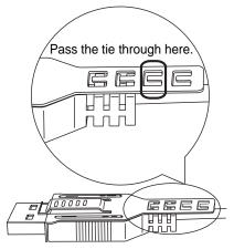
(3) As shown, pass the tie through the clip hole. Next, turn the tie and pass it slightly through the head so that the USB cable can pass through the center of the tie loop. The clip will be lightly attached to the USB cable.
