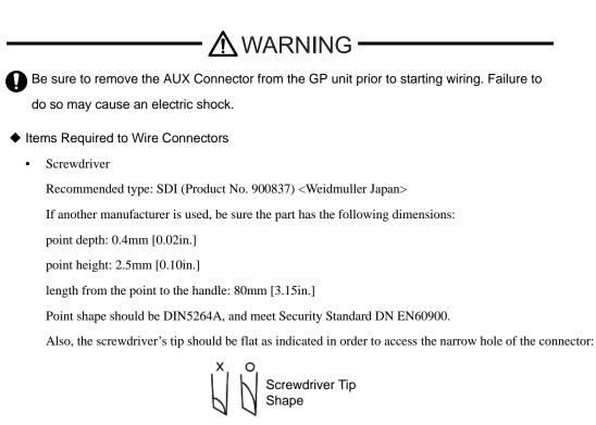
The connectors are a spring clamp type. Use the following procedure to connect the wires to the connectors.
