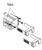
(2) Attach the USB Holder to the USB Host Interface part of the main unit. Hook the upper pick of the USB holder to the attachment hole of the main unit and then insert the lower pick as shown below to fix the USB holder.
