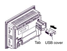
IMPORTANT • Check the up/down orientation of the USB cover to ensure that the USB cable is secured properly.
