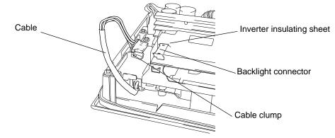
**IMPORTANT** • A hot circuit board chassis can burn you. Be sure the chassis has cooled completely prior to replacing the backlights.
