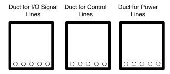
If different wires must be placed in the same duct, separate them with an earthed/grounded divider.
