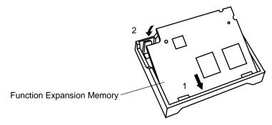
(6) Verify that the Function Expansion Memory is securely attached to the frame.
