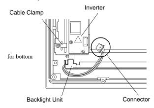
(7) As shown here, push the backlight unit's attachment clip to the right to release the backlight unit.
