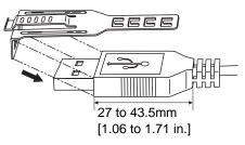
(2) Align the clip and the USB cable connector shell and adjust the position of the holes where the clip is attached. To ensure stability, select the clip-hole position that is closest to the base of the connector shell and that is not making contact with the base.
