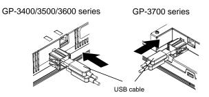
(4) Attach the USB cover to fix the USB cable. Insert the USB cover into the tab of the USB Holder.
