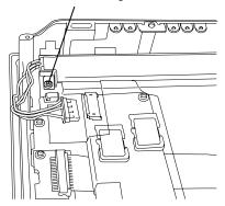
(7) Lift the edge of the Backlight Unit, and remove the unit while sliding it along the groove
