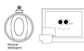
When the display surface or frame become dirty, use a soft cloth moistened with neutral detergent to wipe away any dust or stains.
