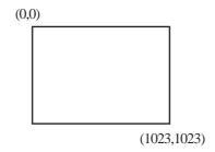
Screen display origin, with resolution of 1024 x 768, is normally at the upper left corner of the screen. Therefore, a software to convert the touch coordinates to display coordinates is needed.
