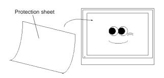
Attach the screen protection sheet when using the FP in extremely dirty or dusty areas.
