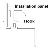
3) Insert each of the fasteners as shown below. Be sure to pull the fastener back until it is flush with the rear of the attachment hole.
