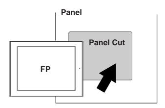
2) Insert the installation fasteners into the FP's insertion slots, at the top and bottom of the unit. (total: 8 slots)
