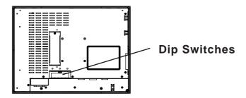
The FP unit's Dip Switches are preset as shown below. These settings are made on the assumption that a Windows® compatible computer is used.
