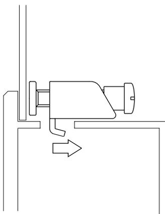
3) Insert each of the fasteners shown below. Be sure to pull the fastener back until it is flush with the rear of the attachment hole.
