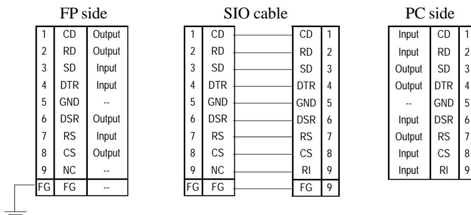
Signal names for the FP's SIO interface are designed to match the same pin order as the SIO interface on a standard PC.
