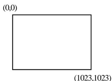
Screen display origin, with resolution of 640 x 480, is normally at the upper left corner of the screen. Therefore, a software to convert the touch coordinates to display coordinates is needed.
