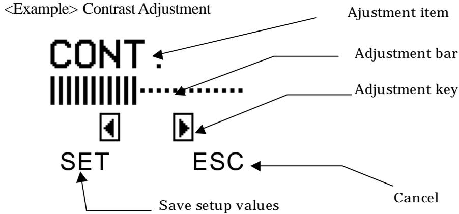
The value for each setting item can be increased or decreased by pushing the adjustment key.
