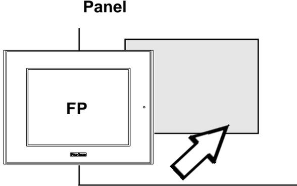
1) Insert the FP into the panel cut out, as shown here.
