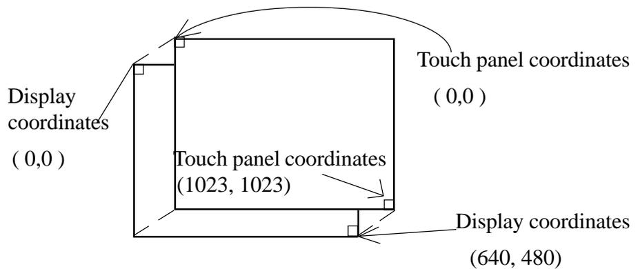
\* The touch panel coordinates are converted to the display coordinates when "FPATPH.EXE" is activated.
