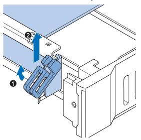
4 Remove the slot cover from the PCIe Drawer.
