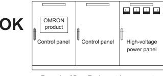
**Example of Poor Equipment Arrangement**
