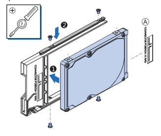
**5** Insert the bracket with the drive into slot B of the Box PC. Ensure the bracket is completely in the Box PC with an extra push.
