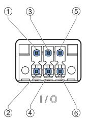
The pin layout represents the I/O connector on the Box PC. Pin details of the I/O Connector:
