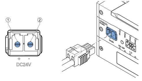
The pin layout represents the power connector on the Box PC.
