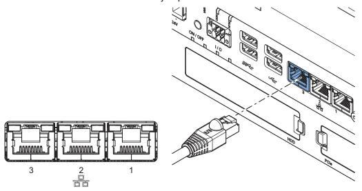
The view represents the Ethernet connector on the Industrial Box PC.
