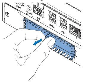
4 Insert the drive cover in the drive bracket slot 1 and move it down 2 so that it locks in the drive bracket.
