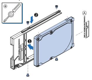
8 Insert the bracket with the replacement drive into the correct slot of the Box PC. Ensure the bracket is completely in the Box PC with an extra push.
