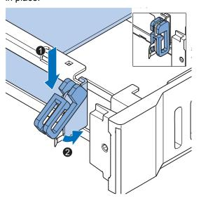
9 Slide the Card Support • so that it supports the side of the PCIe Card.
