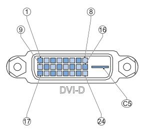
The pin layout represents the DVI connector on the Industrial Box PC. Pin numbers increase from left to right for every row.
