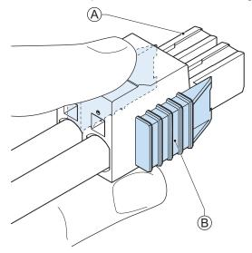
Do not push the orange sliders <sup>(B)</sup> in the direction of the Box PC because this will unlock the connector.
