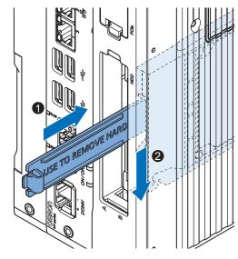
**5** Remove the drive bracket from the Box PC using the drive cover.
