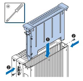
**9** Remove the PCIe cover if the PCIe Card has external connectors.
