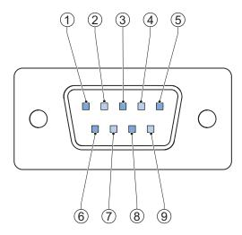
The pin layout represents the RS-232 connector on the Box PC.
