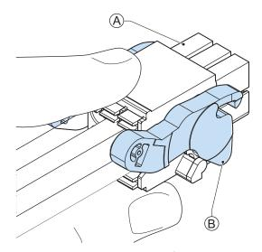
Do not tilt the orange levers <sup>(B)</sup> because this will unlock the connector.
