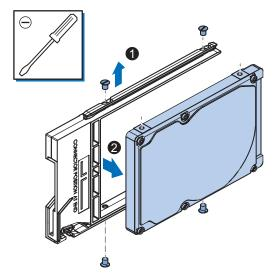
**7** Align the connectors of the replacement drive as shown A on the bracket. Then insert the replacement drive 1 in the bracket and insert the 4 mounting screws 2. Tighten these screws with a torque of 0.35 N·m.
