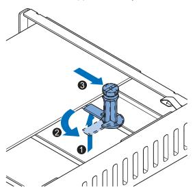
**5** Pull the middle of the Card Clip to unlock it and remove it from the PCle Drawer.
