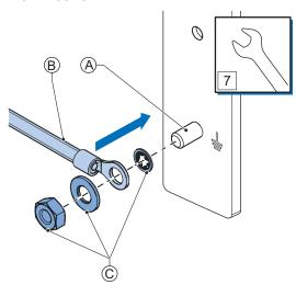
Mount the ground connection wire B to the functional ground terminal A using the washers and nut C. Tighten the nut with a torque of 1.2 N·m max.
