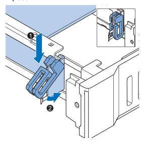
Slide the Card Support of so that it supports the side of the PCle Card.
