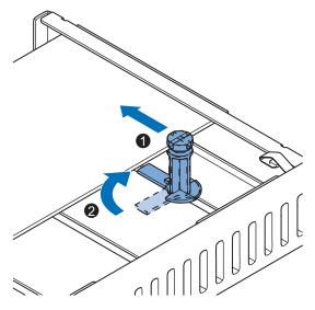
Ensure the Card Support contacts the PCle Card with the small groove so that there is support below and above the PCle Card.
