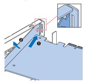
Ensure the PCIe Card is inserted into the correct opening.
