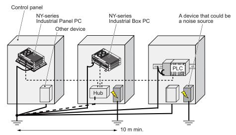
(b) Connecting devices and noise sources to a common earth electrode
