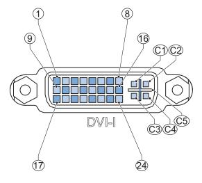
The pin layout represents the DVI-I connector on the Industrial Box  ${\sf PC}.$
