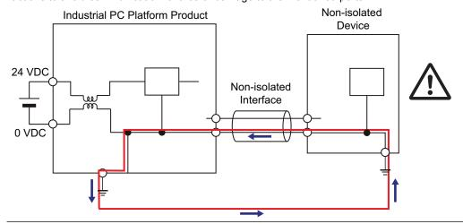
Never ground the 24 VDC side of the power supply. This may cause a short circuit.
