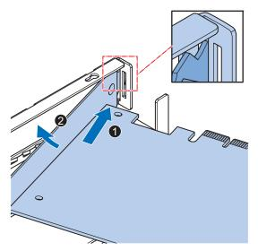
Ensure to insert the PCIe Card in the correct opening.
