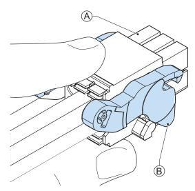
Tilting both levers <sup>(B)</sup> will release the I/O connector <sup>(A)</sup> from the Box PC.
