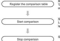
Register the comparison table with the CTBL (COMPARISON TABLE LOAD) instruction. Specify the interrupt tasks to be started in this step.
