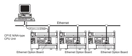
Executing, from the host computer, FINS commands with UDP/IP or TCP/IP headers enables various control operations, such as the reading and writing of I/O memory between PLCs, mode changes, and file memory operations.
