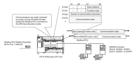
Modbus-RTU commands can be sent simply by turning ON a software switch after setting the Modbus slave address, function, and data in the DM fixed allocation words for the Modbus-RTU Easy Master. The response when received is automatically stored in the DM fixed allocation words for the Modbus-RTU Easy Master.
