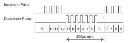
• Cycle time exceeded error occurs when using target matching When using target matching, if the encoder input values change fast due to vibration, the direction changing may be at a high frequency, cycle time exceeded error may occur as a result. At this time, take measures to stabilize the encoder inputs or use range comparison.
