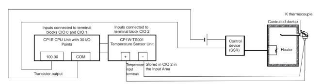
• A K thermocouple is used for the temperature input. Use a CP1W-TS001 Temperature Sensor Unit (thermocouple input).
