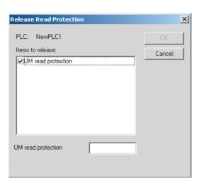
2 Enter the registered password. If the password is incorrect, the message shown on the right will be displayed, and protection will not be released.
