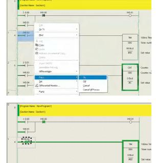
The input bit will be force-set. A symbol indicating the force-set status will be displayed at the input condition.
