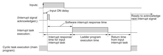
The time from when execution of the input interrupt task is completed until execution of the cyclic task is resumed is  $24 \ \mu s$ .
