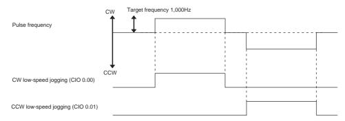
The example shows jogging with acceleration and deceleration executed using an ACC instruction. It is used for high-speed jogging.
