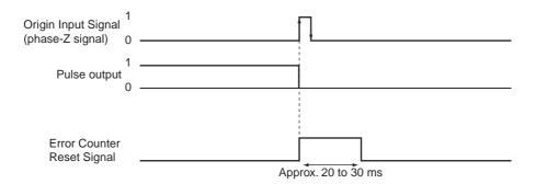
Though the Origin Proximity Input Signal is received, the signal will be ignored and the motor will begin decelerating from the origin search high speed to the origin search proximity speed. In this operating mode, the motor will stop at the Origin Input Signal after deceleration is completed.
