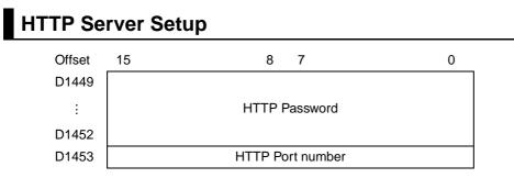
If the password for accessing the Ethernet Option Board's Web page is forgotten, find out it in this area. It is written in ASCII format.
