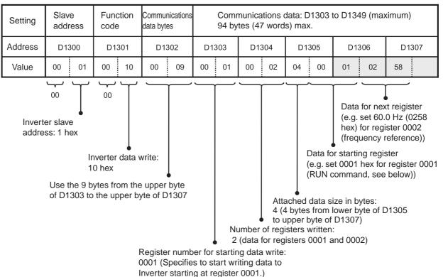
Serial Option Port or Built-in RS-485 Port: Command
