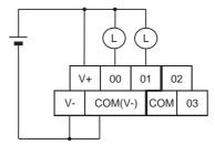
Although V- and COM(V-) are connected internally, also wire them externally.
