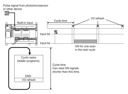
The pulse widths of quick-response input signals must meet the following conditions.
