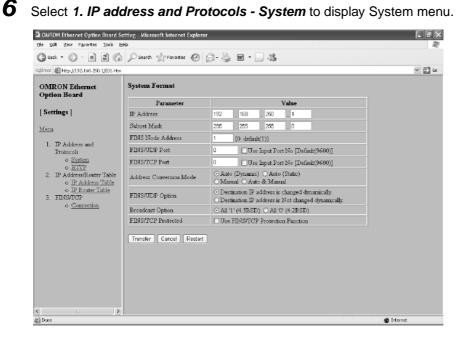
7 Make the required settings (i.e., the IP address in this example).
