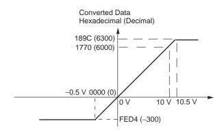
**Note** When the input exceeds the specified range, the AD converted data will be fixed at either the lower limit or upper limit.
