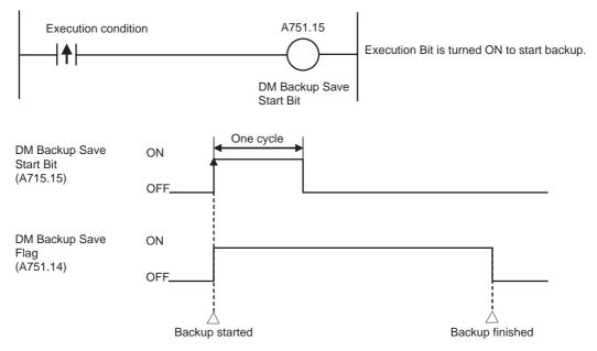
When the saving operation has been completed, A751.14 (DM Backup Save Flag) will turn OFF.
