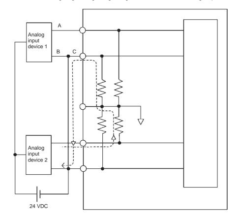
**5** Refer to the following diagram regarding wiring disconnections when voltage input is being used.
