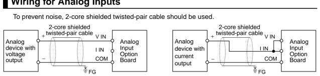
Wiring for Analog Inputs
