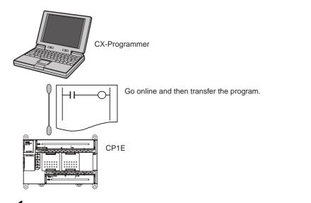
**1** Open the project containing the program to be transferred from the CX-Programmer.
