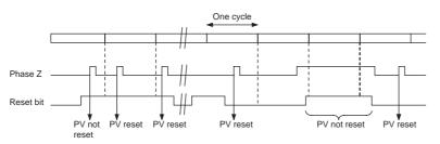
Note The phase-Z signal cannot be used if an incremental counter is specified. Only a software reset can be used.
