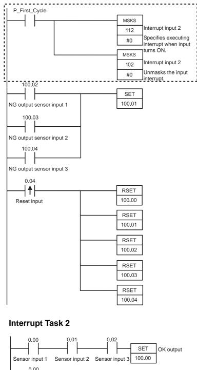
The MSKS instruction is used to specify an interrupt when the input turns ON and then it is used to unmask the input interrupt.
