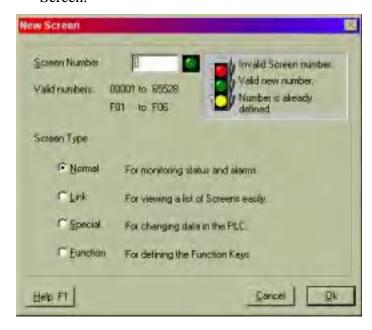
3. Four different types of screens can be selected from the New Screen dialog: Normal, Link, Special, and Function. The following sections will discuss each type of screen. Choose a screen type, enter a screen number, and select OK to launch the Editing Screen dialog.
