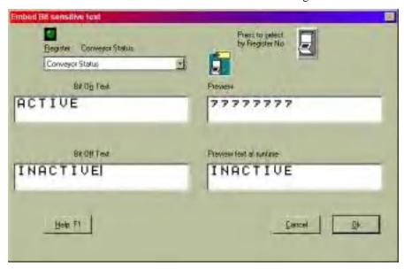
Once the text is assigned to bit values and OK is selected, text placeholders will appear in the display window. These placeholders can be positioned by adding characters before the placeholders. In this case, spaces were added at the far left of the second line to center the text.
