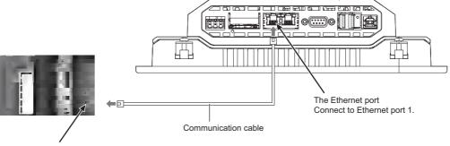
The internal Ethernet/IP port
