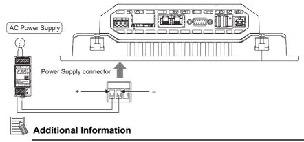
This guide uses the Power Supply Unit, S8VS-06024. However, you can use any Power Supply Unit that satisfies the specifications.
