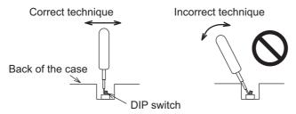
The DIP switch may break if it is levered with a tool against the case as shown in the figure.
