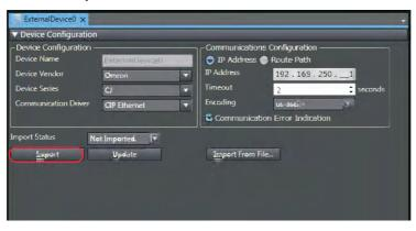
**3** The global variables of the CJ-series PLC are transferred and registered as device variables.
