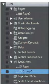
**3** Open the added Resources table, and register a text string to display on an object.
