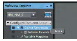
2 Select Add - ExternalDevice. The device is added as ExternalDevice, where is a serial number starting from 0.
