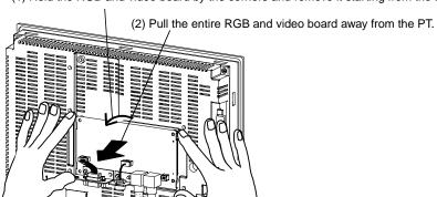
(1) Hold the RGB and video board by the corners and remove it starting from the top.
