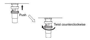
(2) After unlocking the BNC socket, pull it out.
