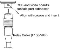
The socket locks into place when it is inserted.
