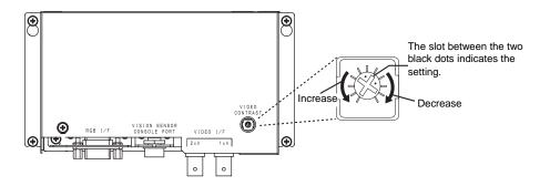
\* The image may be distorted if the contrast adjustor is turned too far. When that happens, turn the adjustor in the opposite direction until the distortion is eliminated.
