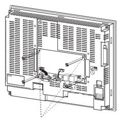
Remove the screws securing the four corners.
