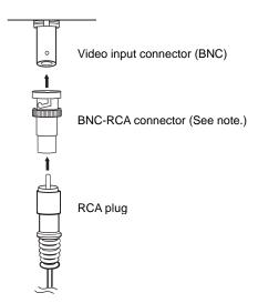
\* The BNC-RCA connector is not provided with the RGB and Video Input Unit (NS-CA002).
