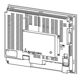
(6) Slide the cover downward and tighten the screws.
