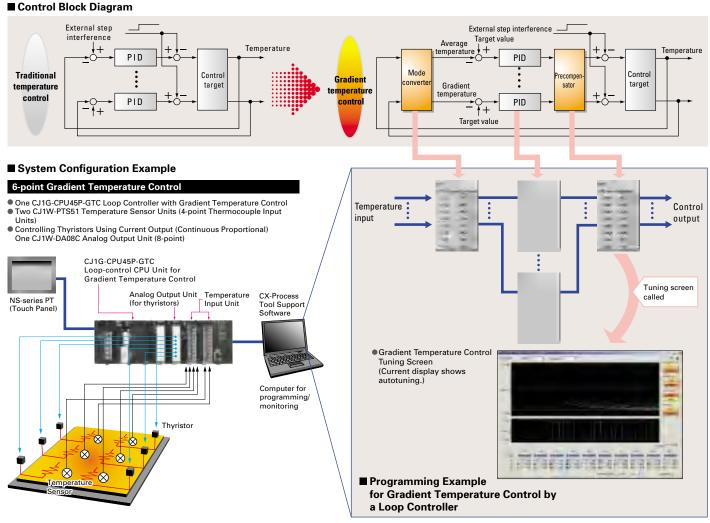
Note: Real programs require gradient SP mode conversion blocks to input settings to each PID block.
