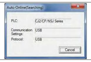
6 Confirm that the CX-Programmer and the PLC are normally connected online.
