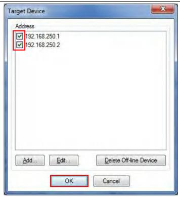
The device parameters are uploaded. When uploading is completed, the dialog box on the right is displayed. Check the contents and click the **OK** Button.
