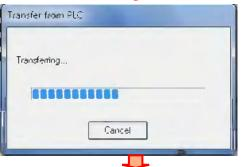
When the transfer is completed, the Transfer Results Dialog Box is displayed.
