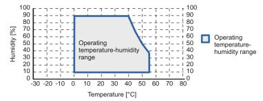
The ambient operating temperature specifications do not depend on the mounting angle, orientation or display size.
