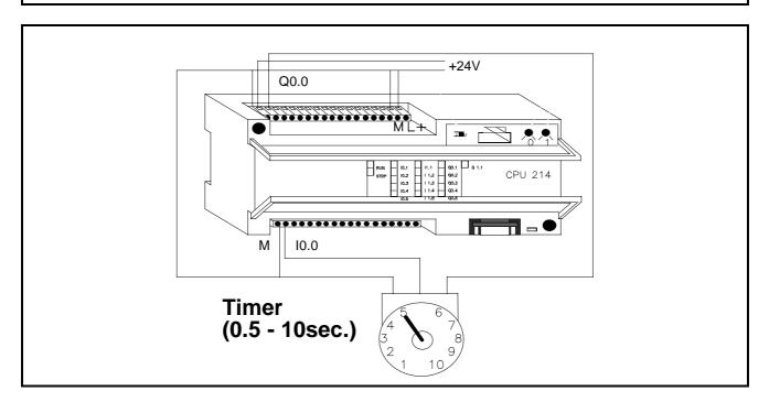
Figure 43.1 Connection of the Timer to the S7-200 PLC
