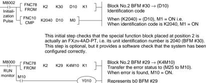
This step provides optional monitoring of the FX2N-4AD-PT Error Buffer Memory (#29). If there is an Error on the FX<sub>2N</sub>-4AD-PT, bit b0 of BFM #29 will be set on. This can be read by this program step, and output as a bit device in the PLC (Y010 in this example). Additional Error devices can be output in a similar manner, i.e. b10 BFM #29. (see below)
