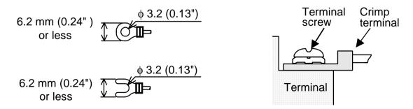
Handle the crimp terminal of the following size when 2 wires are used per terminal.
