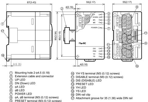
The hardware high-speed counter block is a 2-phase 50 kHz high-speed counter. It is a special function
