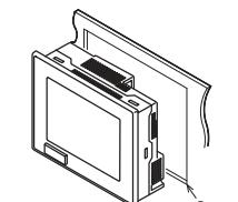
④ Engage the hook of the mounting fitting (supplied) to the unit fixing hole of the GOT and tighten the screw until the GOT is fixed. Please use all four supplied mounting fittings and tighten the mounting screws with a torque of 0.3 to 0.5 Nm.
