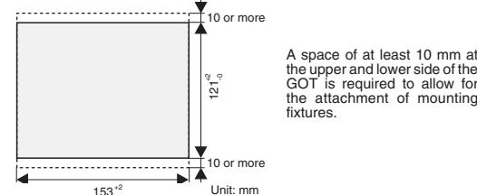
A space of at least 10 mm at the upper and lower side of the GOT is required to allow for the attachment of mounting fixtures.
