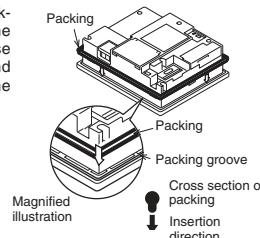
③ Insert the GOT from the front of the panel or the control cabinet into the cut out.
