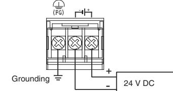
Use 0.75 mm<sup>2</sup> or thicker cables to avoid voltage drop and tighten the terminal screws securely with a torque of 0.5 to 0.8 Nm. Use commercially available terminal ends for M3 screws for connection of the power supply (see figure below).
