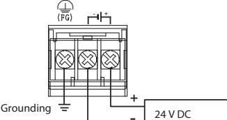
Use 0.75 mm<sup>2</sup> or thicker cables to avoid voltage drop and tighten the terminal screws securely with a torque of 0.5 to 0.8 Nm.
