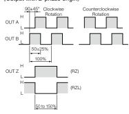
Note: Clockwise rotation when the main body is seen from the axle side is the normal rotation.
